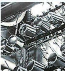
All of our aluminium components are individually loaded onto bespoke titanium pins ready for anodising. Our unique anodising belt process ensures all surfaces of the aluminium are anodised consistently every time.
